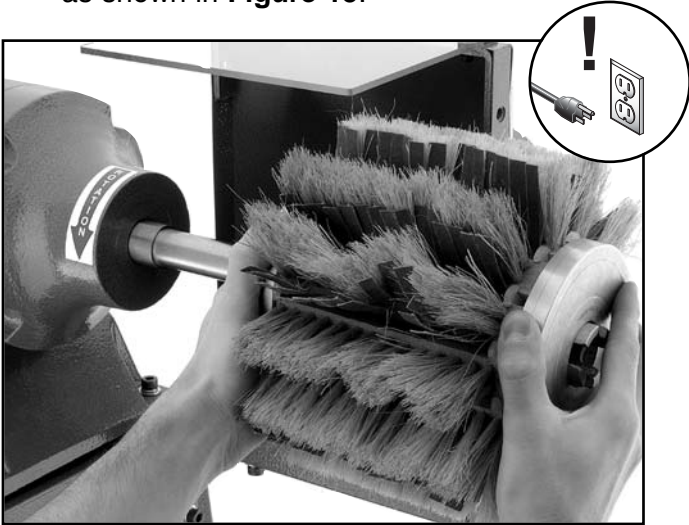
Figure 15. Sliding the flap sander onto the arbor.
